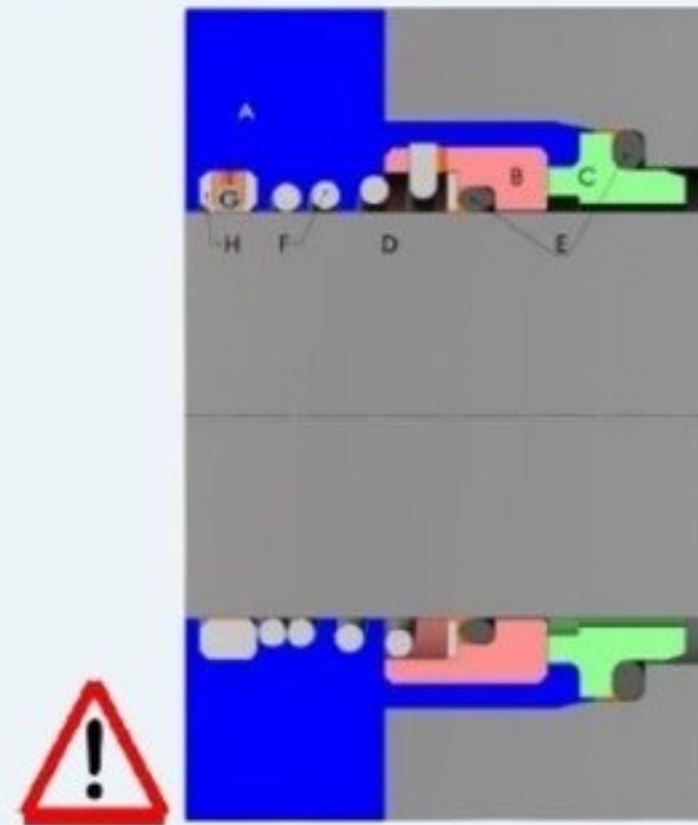
Figure 2. Simple Mechanical seal design, Not hygienic!
